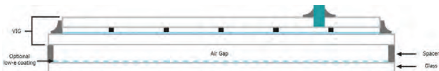
Diagram of a typical hybrid VIG unit—a standard double glazed IGU with air or gas-filled space combined with VIG.
