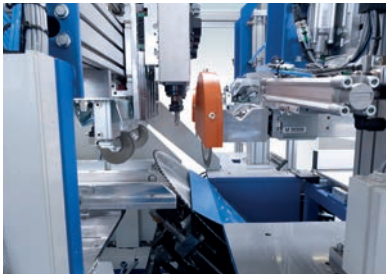
Linear Pro VHC-Cut with notching option
