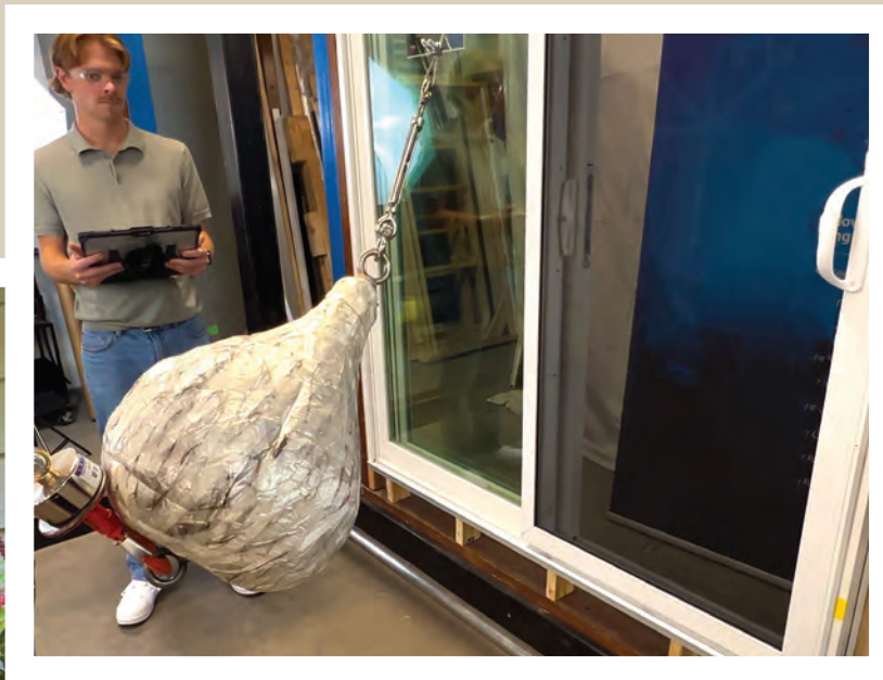
↑ AAMA 1901'S TESTING IS CONDUCTED ON THE SCREEN MATERIAL AND ON THE WINDOW OR DOOR SCREEN ASSEMBLY. ASSEMBLY TESTING SIMULATES REPEATED IMPACT AND FORCED-ENTRY ATTEMPTS, FOLLOWED BY PRYING AND PULL TESTS AT LOCKING POINTS. PHOTO COURTESY OF UHD INNOVATIONS.
